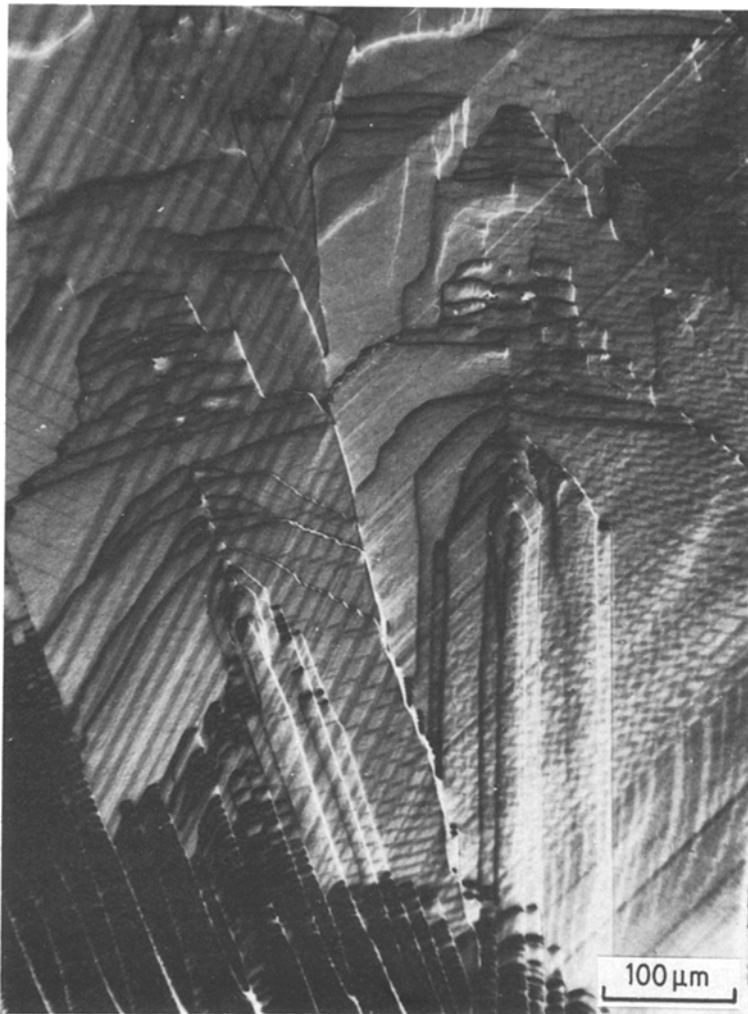
Figure 1 Antiferromagnetic twinning domains on the as-grown (100) surface, photographed by DIM. The dendrite on the left shows predominant two-wall domains and the one on the right shows four-wall domains.
